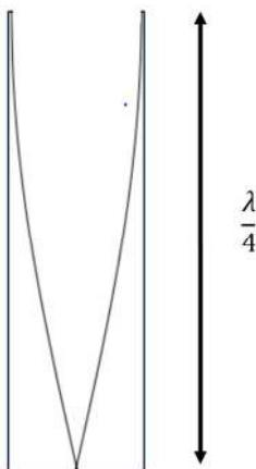
$$\frac{\lambda}{4} = 10 \quad \lambda = 40 \text{ m} \quad \text{so} \quad f = \frac{v}{\lambda} = \frac{320}{40} = 8 \text{ Hz (Answer B).}$$
