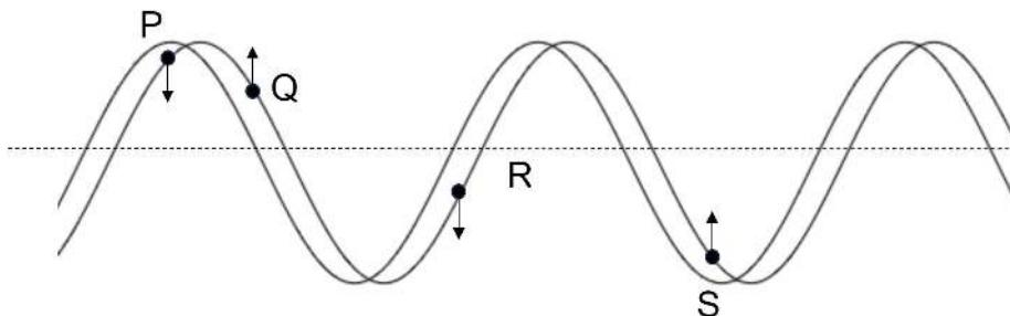
Points Q and S must move up (answer **D**) and points P and R must move down.
