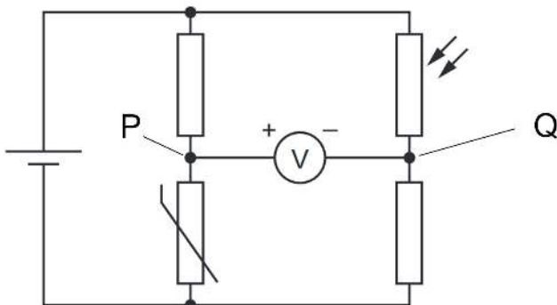
One way to approach this question is to consider the p.d. across P and Q indicated on the circuit diagram. As the temperature increases, the resistance of the thermistor decreases and the p.d. across the thermistor falls – the voltmeter reading will decrease. As the light intensity increases, the resistance of the light dependent resistor (LDR) decreases and the p.d. across the LDR falls – the voltmeter reading will again decrease.
