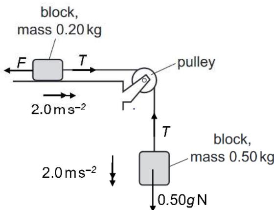
The tension  $T$  in the string acts on both masses as shown. If the friction force acting between the lighter block and the rough surface is  $F$ , then applying  $F = ma$  to both blocks:
