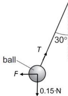
If the tension in the string is  $T$  and the force on the ball due to the air flow is  $F$ , then:
