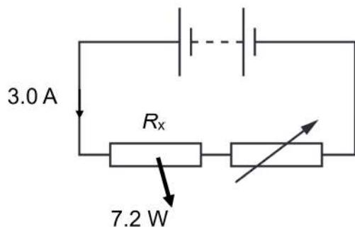
If the resistance of the fixed resistor is  $R_x$ , then using  $P = I^2R$ :
