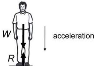
The two forces acting on the man are his weight  $W$  acting downwards and the force  $R$  acting upwards from the floor. Applying  $F = ma$  to the man vertically downwards:
